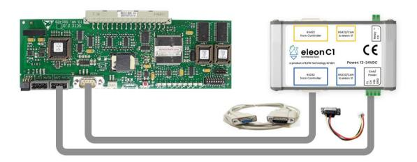
3.4.4. Check the functionality of the D-Sub9 port or XTELE connector & the CAN connector of the CPU board and reconnect the controller and the **eleon C1**. Please press the reset button on the **eleon S1**. The restart of **eleon S1** will trigger another controller connect
