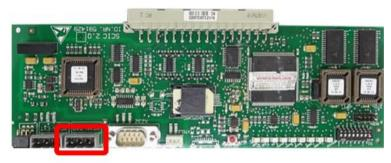
**12.** Use 2 wires to connect CPU board CAN-H & CAN-L to **eleon C1** (green input interface).
