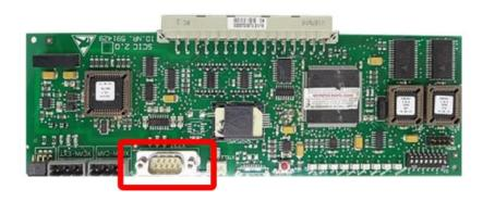
**9.** Use the D-Sub9 cable to connect the CPU board and the **eleon C1** blue labelled connector.
