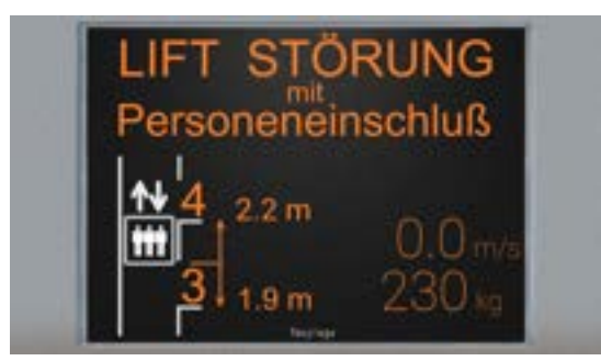
Fig. 1: Display of location and load in case of a failure on a display at the elevator's main entrance.
