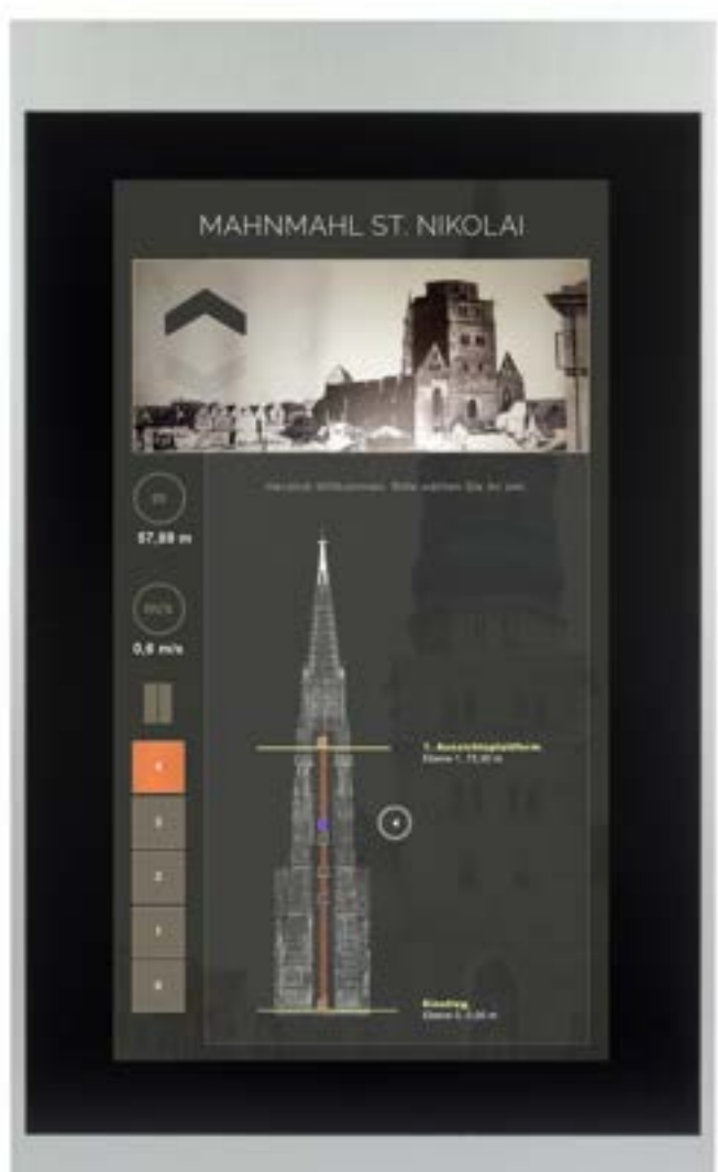
Fig. 7: Example of a position and speed indication, represented as digital value and as true-to-scale graphic.
