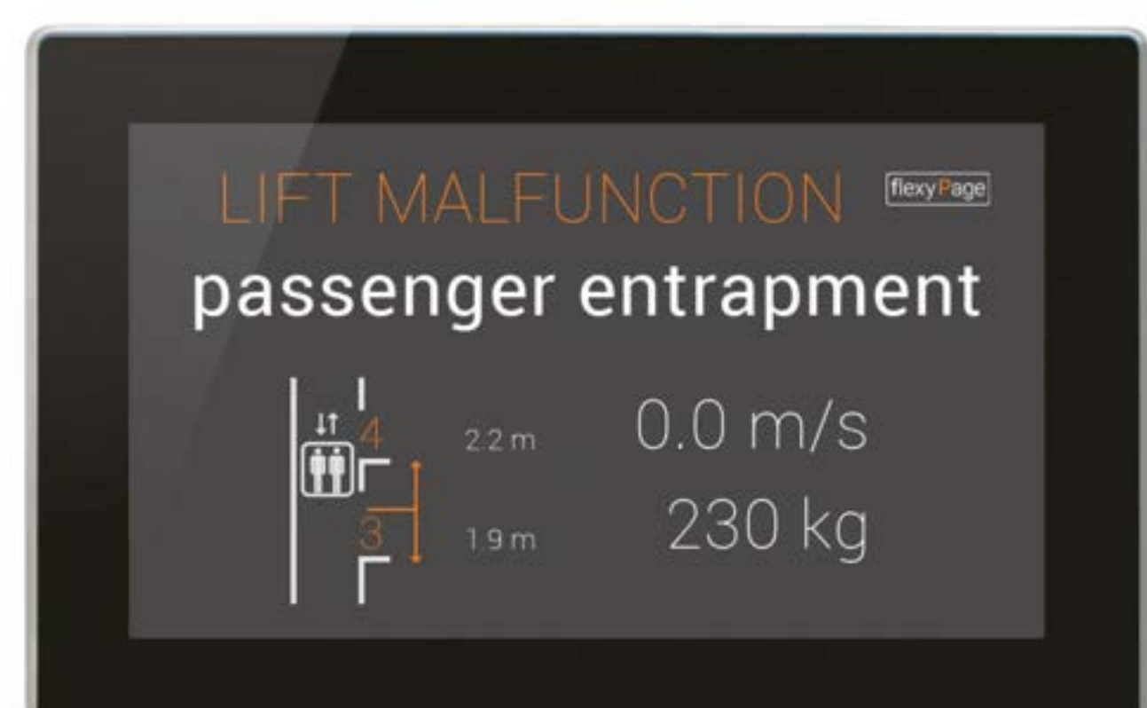
Fig. 5: Emergency note "lift malfunction with passenger entrapment" in a buildings entrance area.
