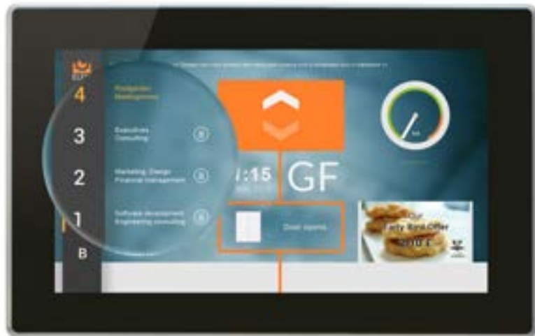
Fig. 3: With flexyPage displays the possibility of access control via a PIN entry is given. Thus, simple access restrictions are realisable.
