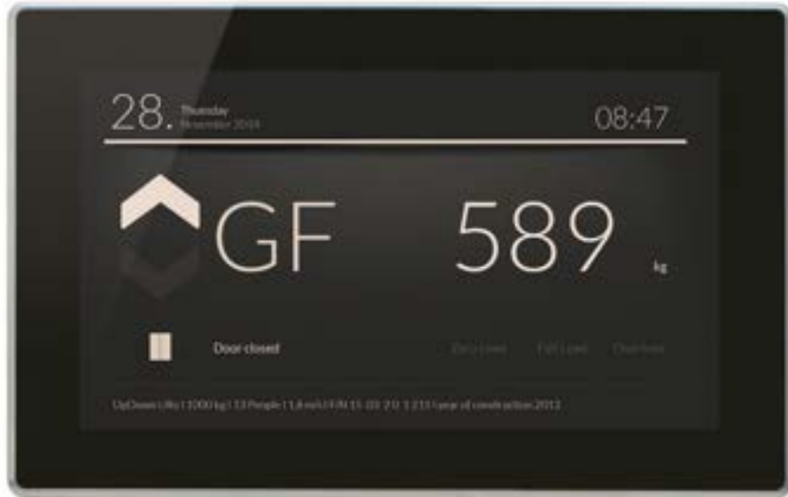
Img.: Depiction of the current load on a display in the lift car.
