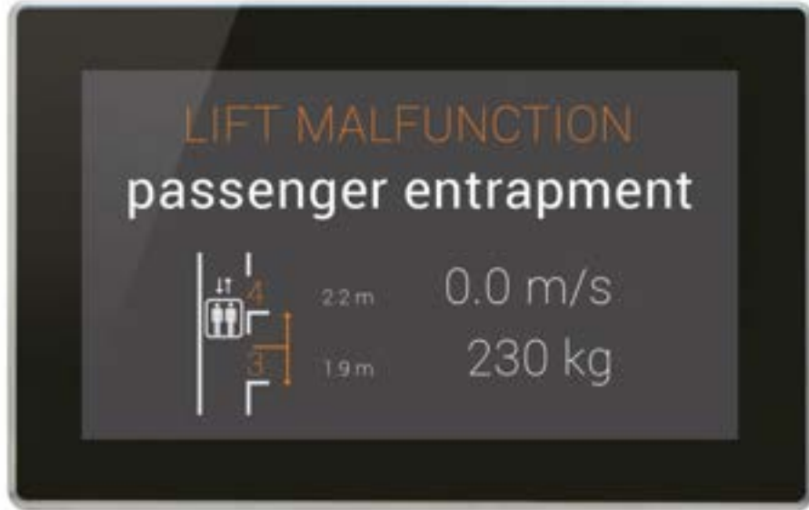
Img.: If data from a position and load measuring sensor are provided via the field bus, this information can speed up the deliverance of trapped persons.
