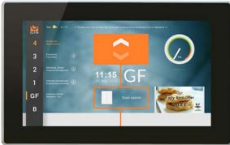
Img.: Depiction of the current load in the cabin through a pointer instrument without the absolute value.
