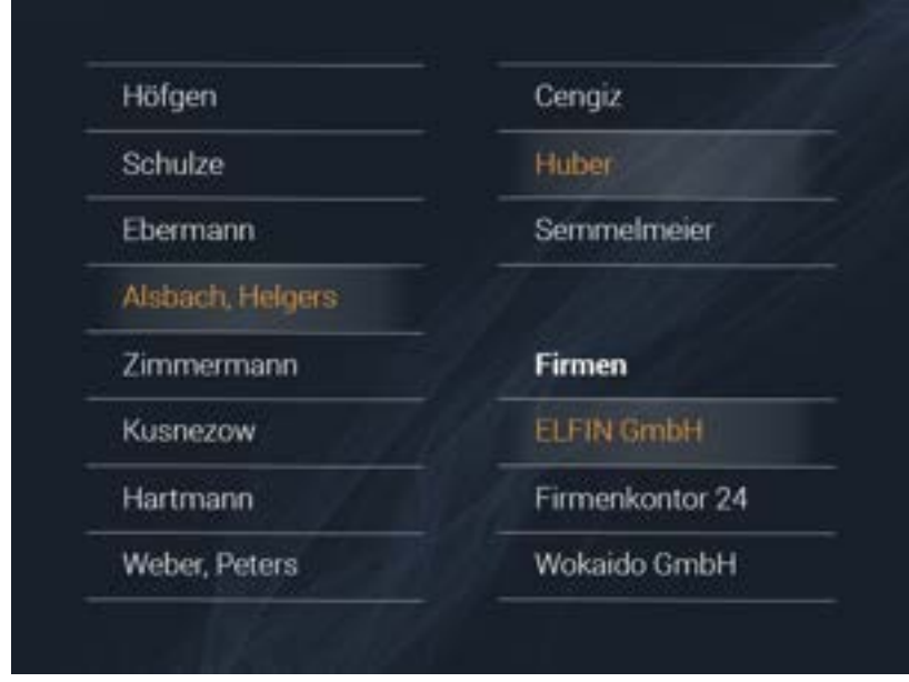
Fig. 2: An individual visualisation of a residents register on a touch screen. The call entry is selected by resident. This is especially helpful, when just the target but not the floor is known.
